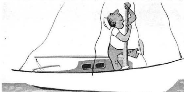
When stays are loose, the result may be a cockeyed or wobbly mast.
