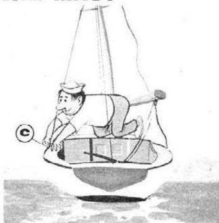
Next, tighten port shroud turnbuckle (C). This will tilt mast over to port.
