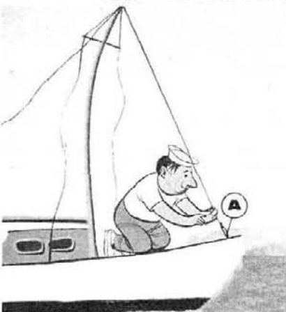
First, tighten jibstay turnbuckle (A). This will bring mast slightly forward.
